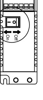
**Please Note: The isolation switch needs to be in the On (↑) position during normal operation**
