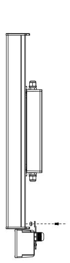
**Step 2** - Proceed to fit sensor bracket onto luminaire by lining up cut out of the bracket to the edge of Lowbay
