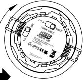
Twist approx 10 deg ensuring all 4 tabs are securely locked in place.
