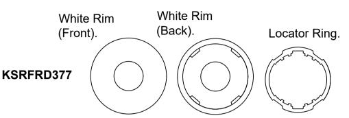
**Void Depth** ØCut out **ØRim Size** Colour Reg'd KSRFRD377 90mm See fitting used info White 100mm 100mm - 120mm | See fitting used info White KSRFRD378 135mm 110mm - 150mm See fitting used info White KSRFRD379 170mm
