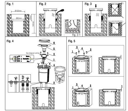
**Decking Fitting -** If fitting this product in decking subject to foot traffic then we would recommend that CFL or LED bulbs are used. If a halogen lamp is required then a 20W lamp should be fitted.
