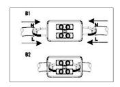
5. Please connect the wires to the LED driver and ensure that the wires are connected into the wiring circuit according to current and relevant wiring regulations.
