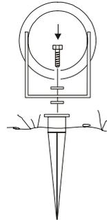
5. If securing into the ground, affix the unit to the spike accessory (included), and firmly push the luminaire assembly into the ground.
