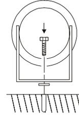
4. To secure the luminaire to a surface, prepare the surface to receive the unit. Use the appropriate method of securing the luminaire according to the substrate it is being fixed to. Use the hole on the mounting bracket to secure the item onto the surface.
